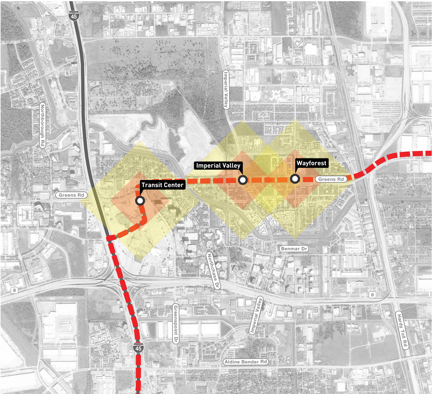
Figure 1.17 BRT Station Placement Greenspoint Mall Site This map is showing recommended station locations balance spacing, access, and land-use considerations. Orange shading represents a quarter-mile walkshed and yellow represents a half-mile walkshed, both based on a conceptual orthogonal street grid.
