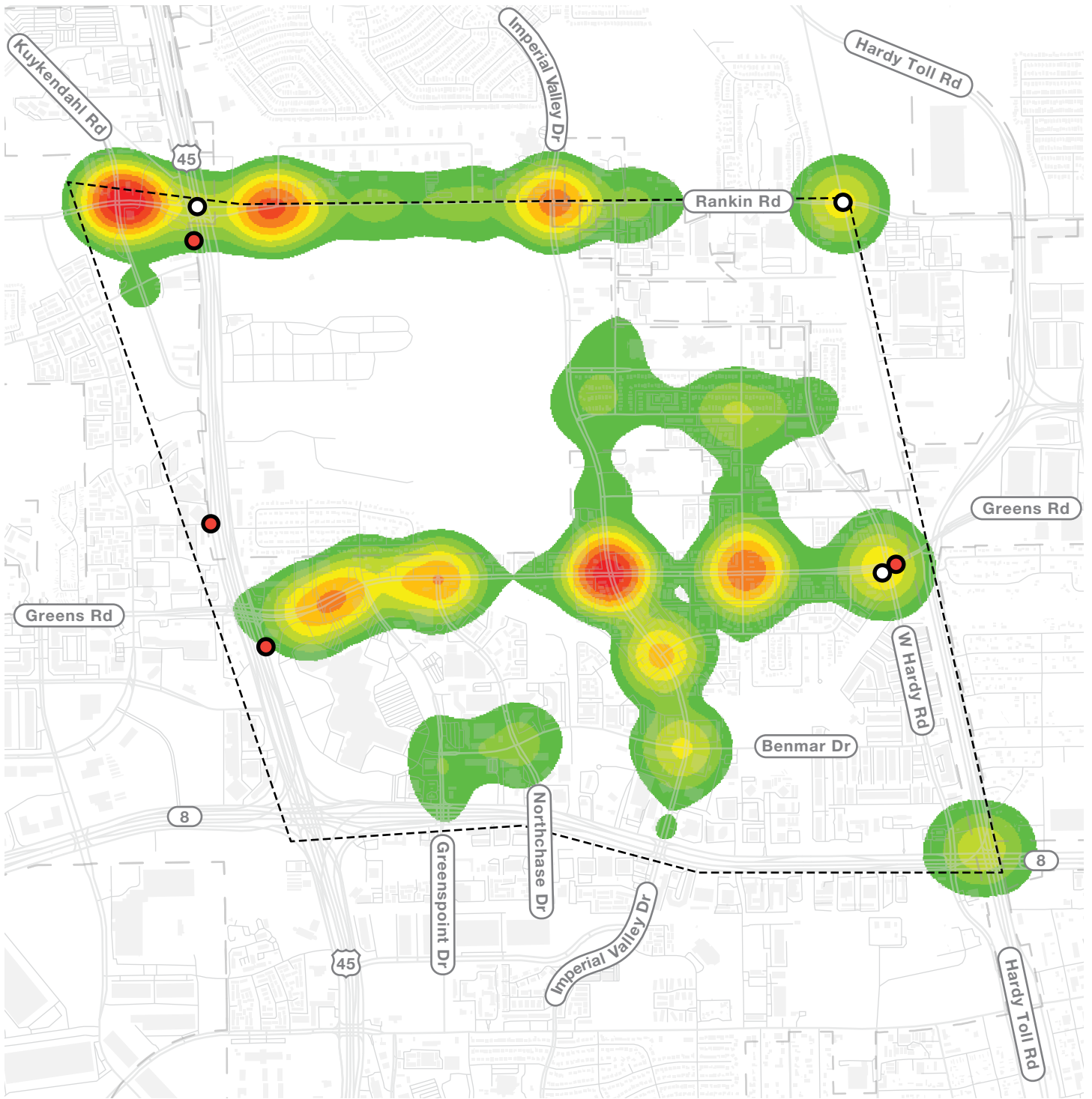
Figure 2.14 Crash Density of All Crashes Wide, straight roads with high volumes – which in this case includes Greens Road and Imperial Valley Drive – often correlate to a higher volume of crashes.
